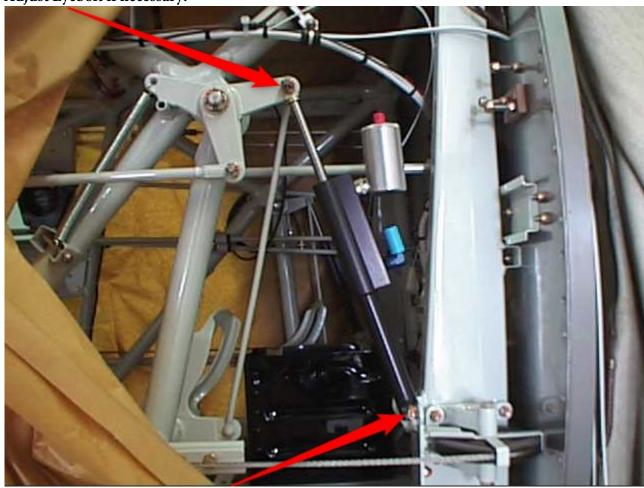
AN4-25A Bolt, do not overtighten. Master cylinder must be free to pivot.
